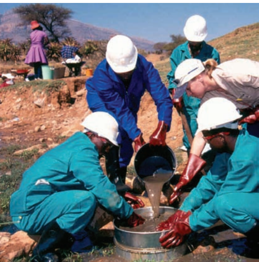
Above: Sediment sampling from a stream - an early part of the search for clues to minerals.
