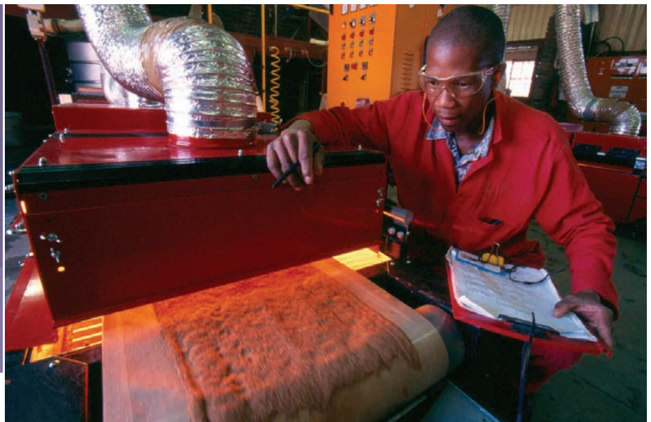
A technician dries mineral samples in a testing laboratory.
